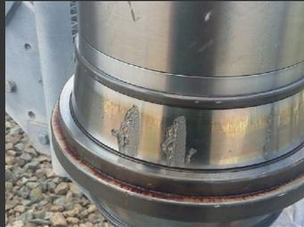
High speed shaft bearing damage detected using ecoCMS
